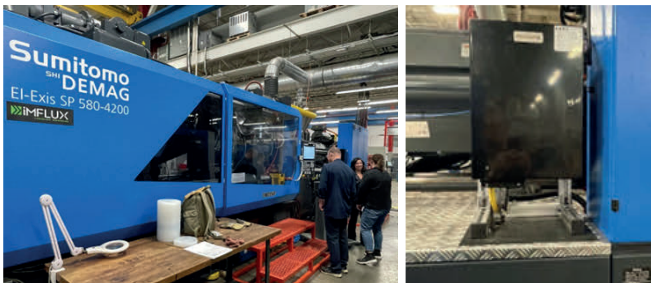
StackTeck Test Machine Equipped with iMFLUX Control Unit (at right)
