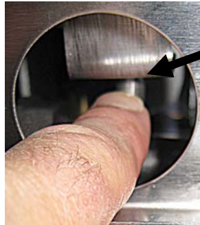
Filter Pump Reset Switch
