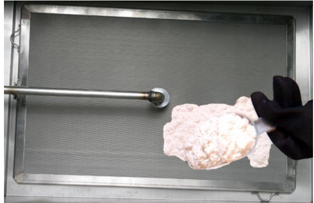
Applying filter powder to filter-leaf.
