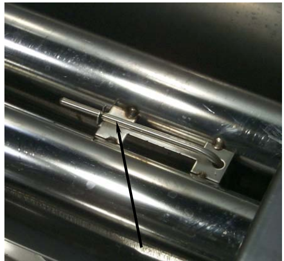
Electronic thermostat probe in frypot (arrow).
