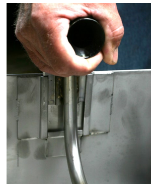
Carefully remove the filter leaf assembly.
