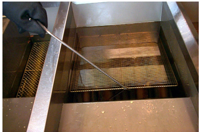
Removing support grid from fry vessel prior to filtering.
