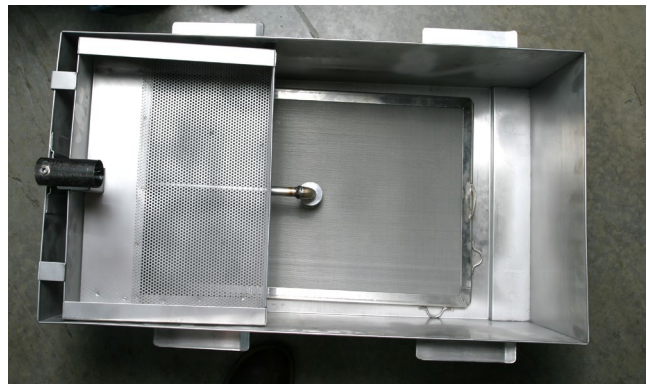
Crumb screen properly placed in filter pan.
