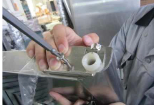
G. Assemble stopper plate in original positions.
