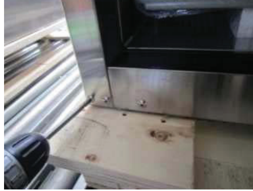
C-2. Disassemble bottom hinge (left).
